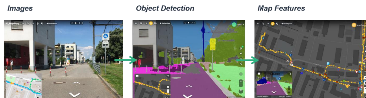
Figure 30: Processing steps of Mapillary's object recognition algorithms (Source: image captures from Mapillary (2021)).
