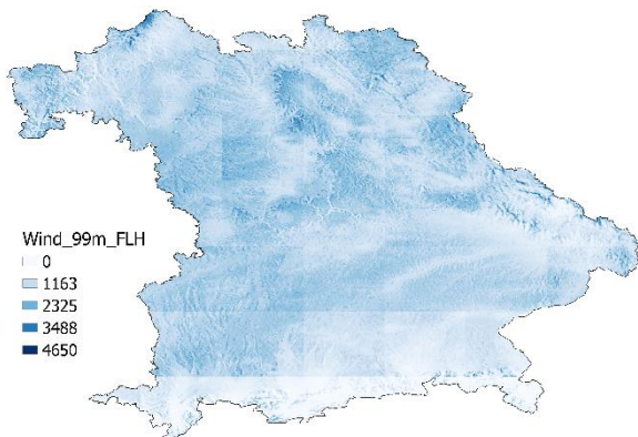
Figure 5: FLH for onshore Wind using 99m high turbine
