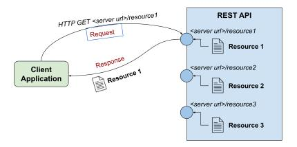
Figure 3.1: General structure of the client-server relationship using a RESTful API.
