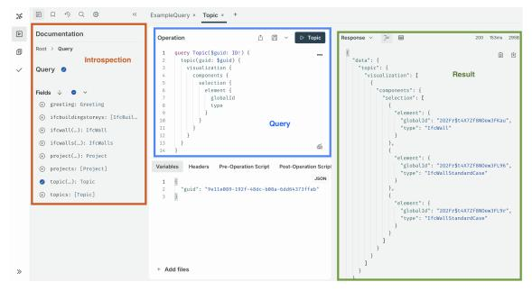
Figure 5.7: Dedicated client to test and explore the GraphQL endpoint.
