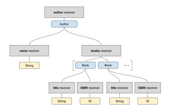
Figure 3.6: "Resolver Chain" or "Resolver Tree" originating from the query defined in 3.6.
