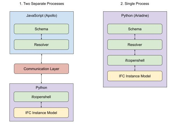
Figure 5.5: Two possible application designs depending on the choice of frameworks and software tools.
