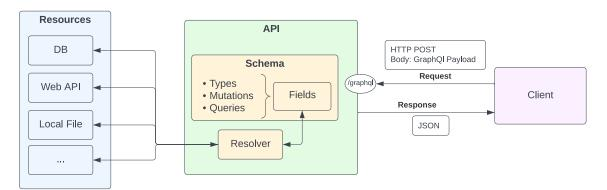
Figure 3.4: Structure of a GraphQL API.
