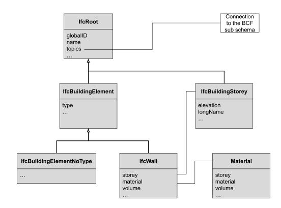
Figure 5.3: Simplified depiction of the GraphQL schema representing the necessary information from the IFC data model.
