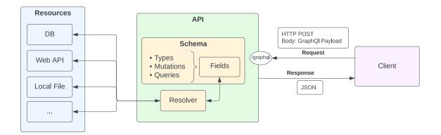
Figure 4.2: API architecture using a classical GraphQL implementation with data access through resolver functions.
