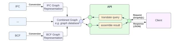
Figure 4.1: API architecture using conversion of data resources into graph representations.
