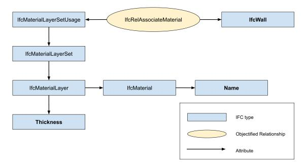
Figure 5.2: Relationship between IfcWall and Material
