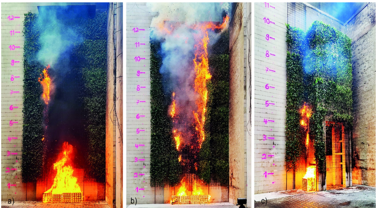
Figure 9: a) Wall test with vital plants (V1); b) Wall test with dried (dead) plants (V2); c) Balcony test with fire exposure in the corner with vital plants (V6)
