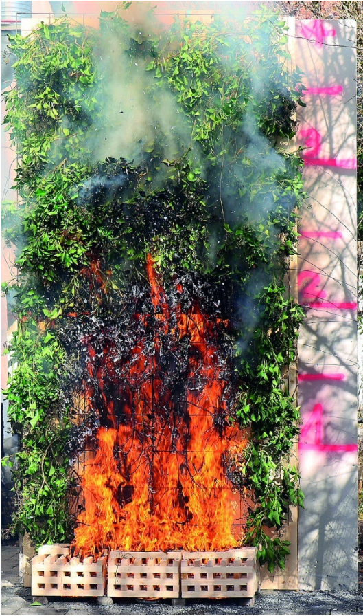
Figure 6: Photo documentation of the fire test (Test 3) with wooden and green façade in the 3rd test minute
