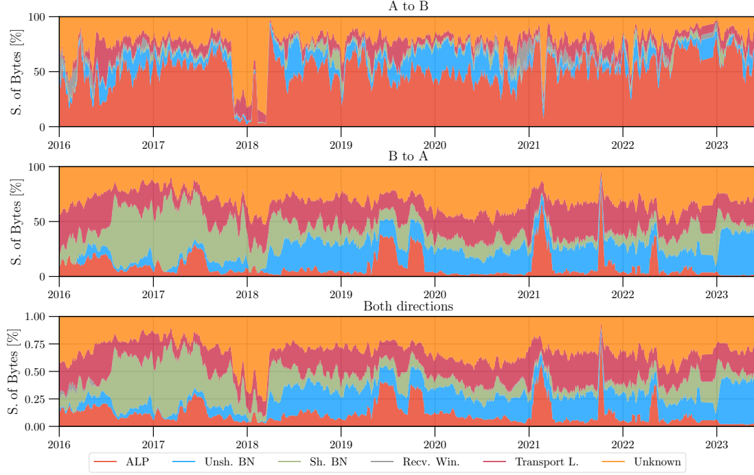
FIGURE 3.12: Shares of transmitted bytes per trace. Data is uniformed with a sliding window of 14 traces.
