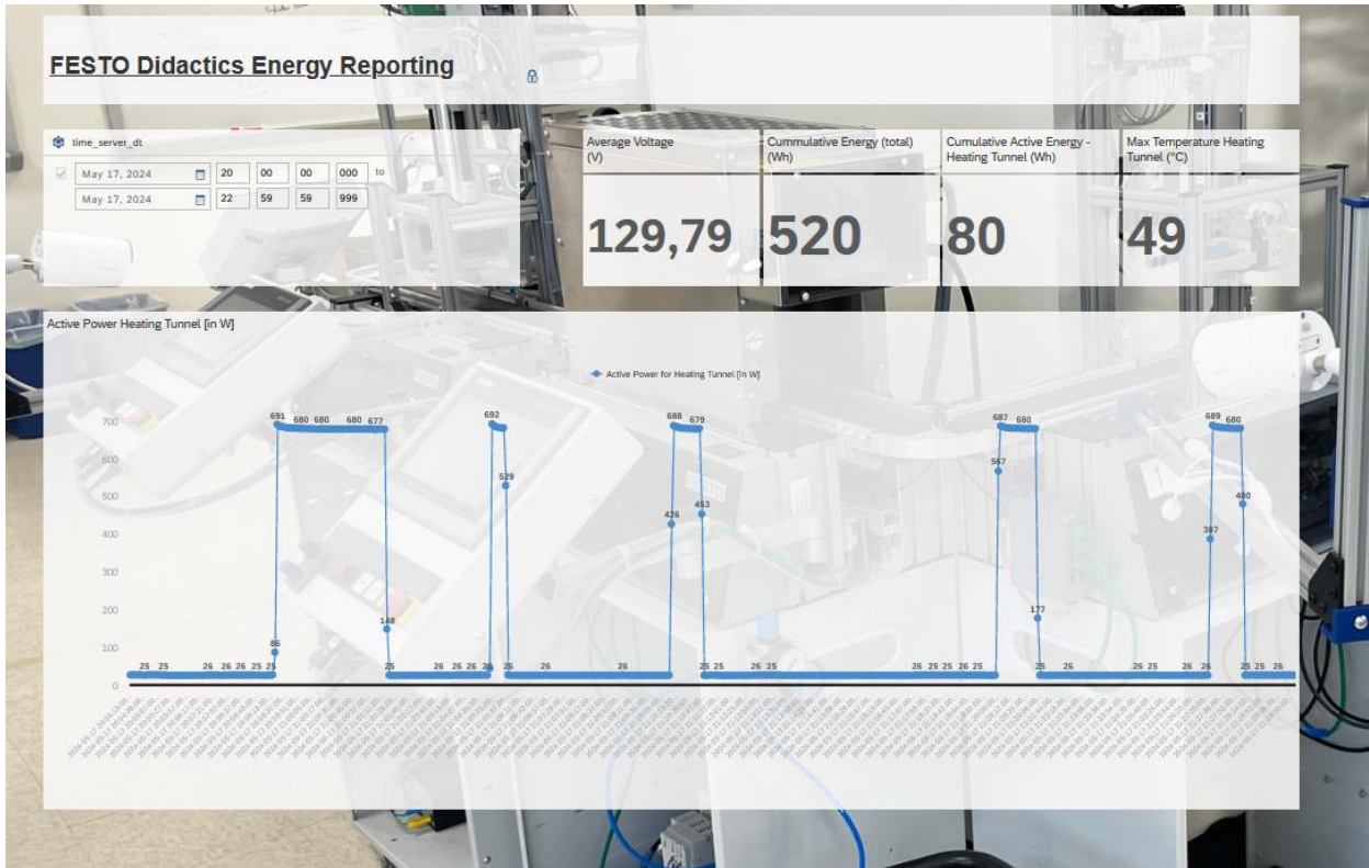
Annex 2: Reporting for energy consumption of the heating tunnel workstation and the total energy consumption of the FESTO® Didactics system
