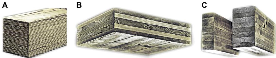
**Figure 4.** Examples of EWPs for structural applications: **(A)** Wood Veneer Composite (WVC) beam. **(B)** Cross-laminated Timber (CLT). **(C)** Glue Laminated Timber (GLT) – two beams of similar strength, the left one of beech hardwood and the right one of spruce softwood, visualizing the difference in beam cross-sections<sup>2</sup>.
