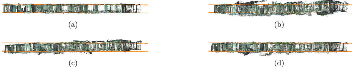
Figure 6.18: Side views of the different maps. (a) ground truth map; (b) map created with synthetic poses of Exp. 1; (c) map after FACaP optimization and (d) after BIMCaP optimization. The BIMCaP result shows better alignment with the real floor and ceiling planes.
