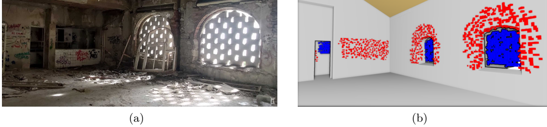
Figure 5.8: Positive and negative differences between the point cloud and the reference BIM model are illustrated as follows: (a) A picture of the real-world scene. (b) Visualization of the detected changes in the form of voxelized clustered meshes with positive differences depicted in blue and negative differences in red. Particularly, it is visible that the windows in the model are smaller compared to the real-world windows.
