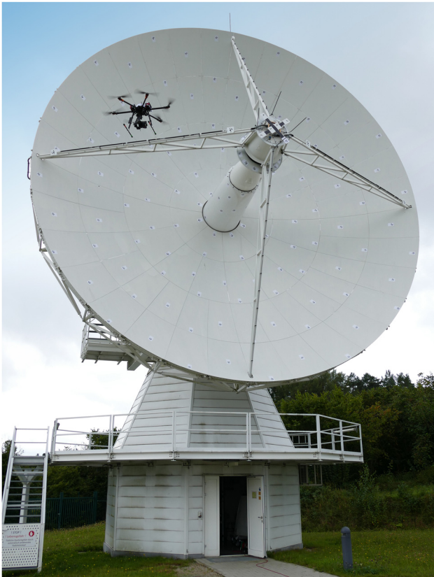
Figure 7: Unmanned aerial vehicle in front of the prepared VGOS radio telescope TTW-2, which is equipped with photogrammetric targets at the receiving unit.
