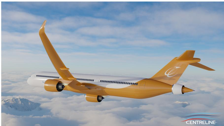
Figure 1.1: Rendering of the turbo-electric PFC developed in the *CENTRELINE* project [7].
