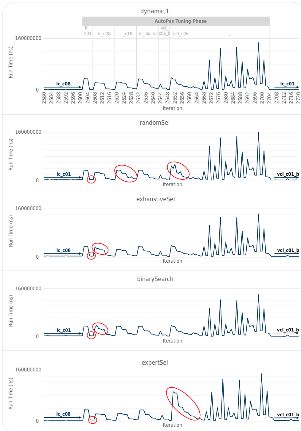
Figure 4.7.: MD-flexible auto-tuned fallingDrop iteration performance. Each graph corresponds to the same tuning phase for all 5 OpenMP schedules.
