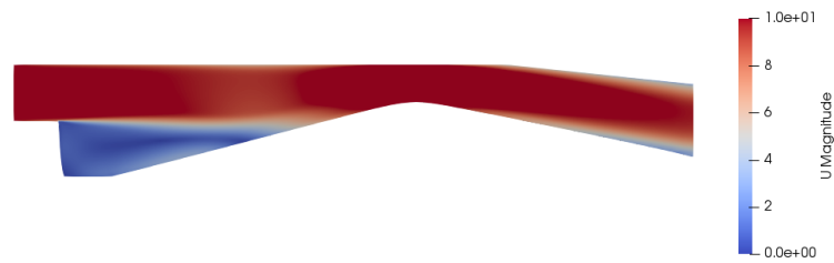
Figure 5.22.: Velocity Contour obtained from simulation of optimized values of the non-stochastic unconstrained optimization problem.
