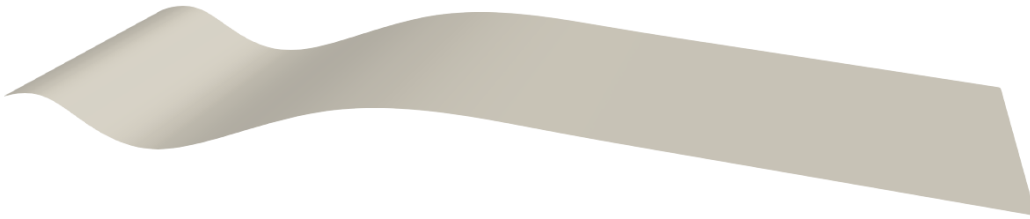
Figure 4.10.: Figure shows the STL curve generated using the Catmull-Clark Subdivision curve.
