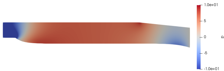
Figure 5.2.: Pressure contour obtained from simulation using initial values from equation 5.2.
