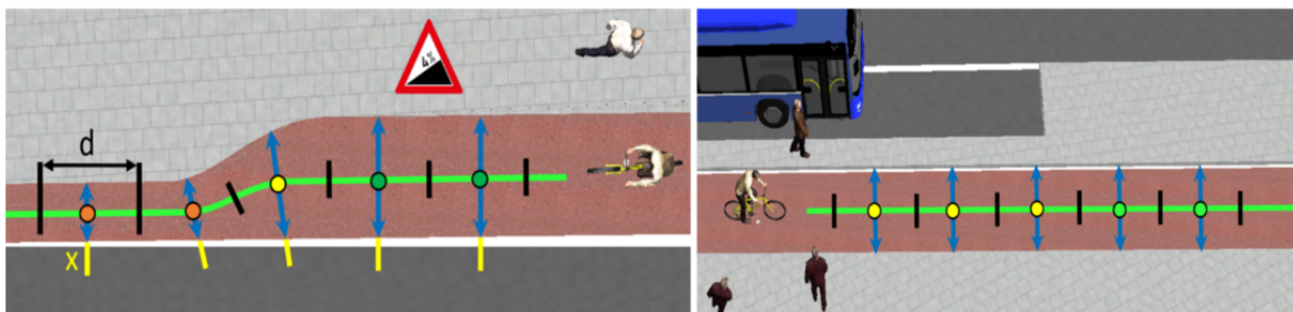
Figure 7.16: Width calculation of bicycle paths at short intervals and determining adjacent surfaces (Beil et al., 2024).
