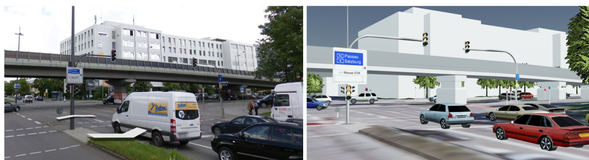
Figure 7.9: Web-based visualization of traffic simulation results for an area around the 'Frankfurter Ring' in Munich with a direct comparison of a Google Street View image.
