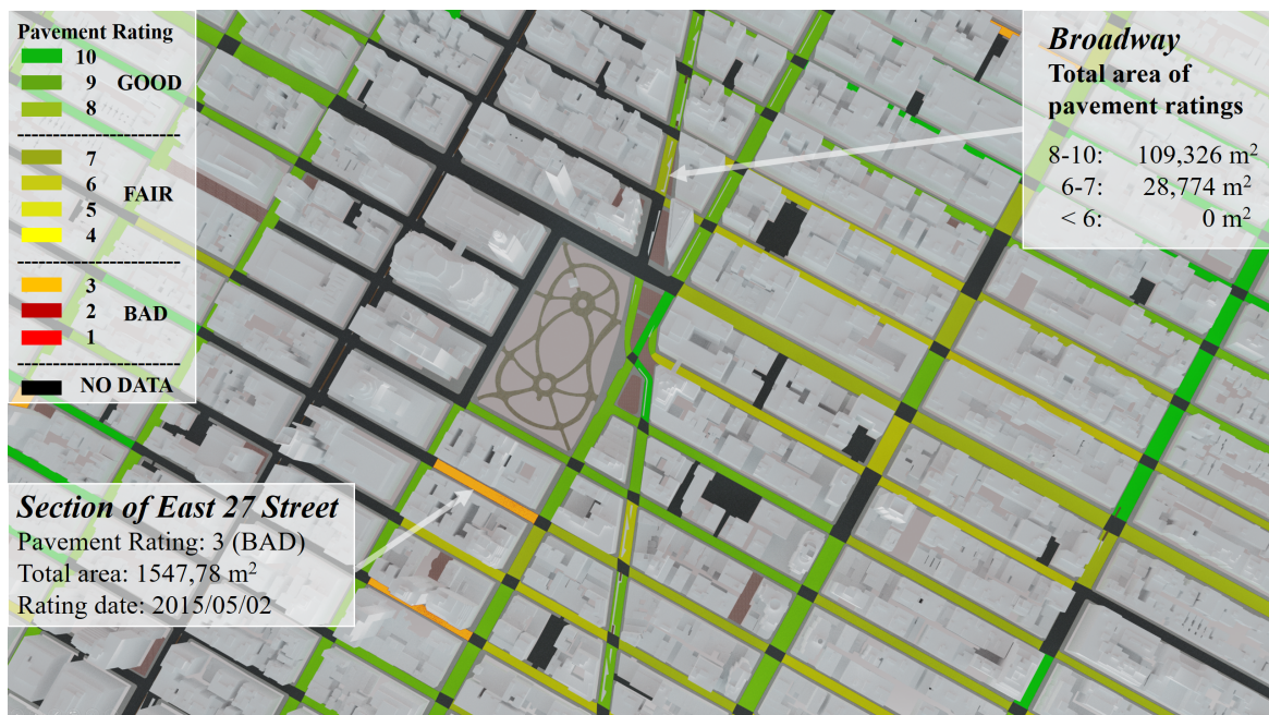
Figure 7.2: Visualization of road pavement ratings of individual sections within a semantic 3D city model of New York City.
