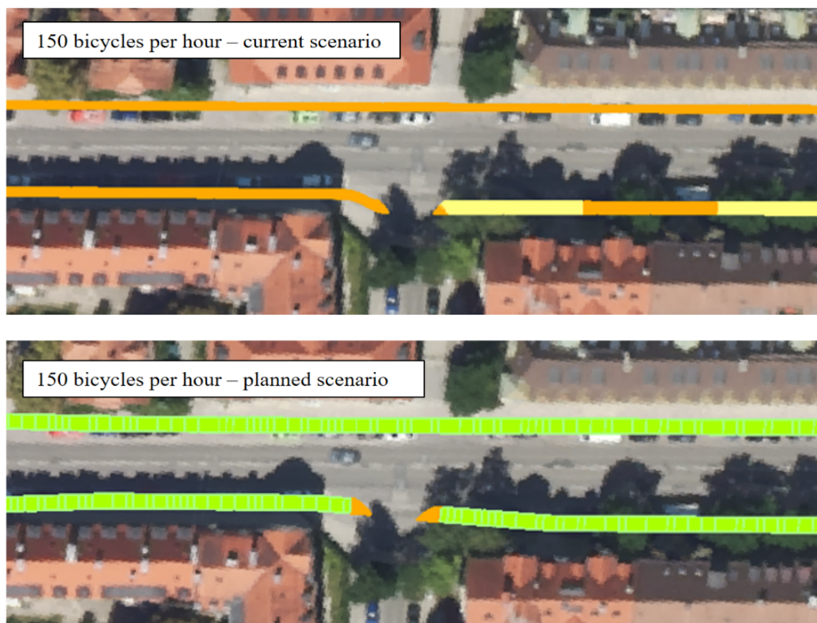
Figure 7.19: Comparison of BLOS values at 150 bicycles per hour of the current state of bicycle paths with a planned scenario (Beil et al., 2024).
