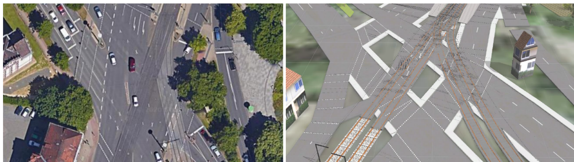
Figure 5.30: Complex intersection of roads and trams. GoogleEarth (left), model generated with the software CityEngine (right) (Gnatz, 2018).
