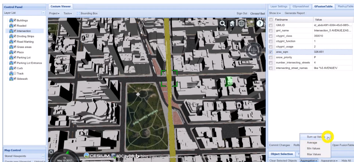
Figure 7.1: Query for all roadbed and intersection areas belonging to 5th Avenue using the 3DCityDB Web Client Pro.
