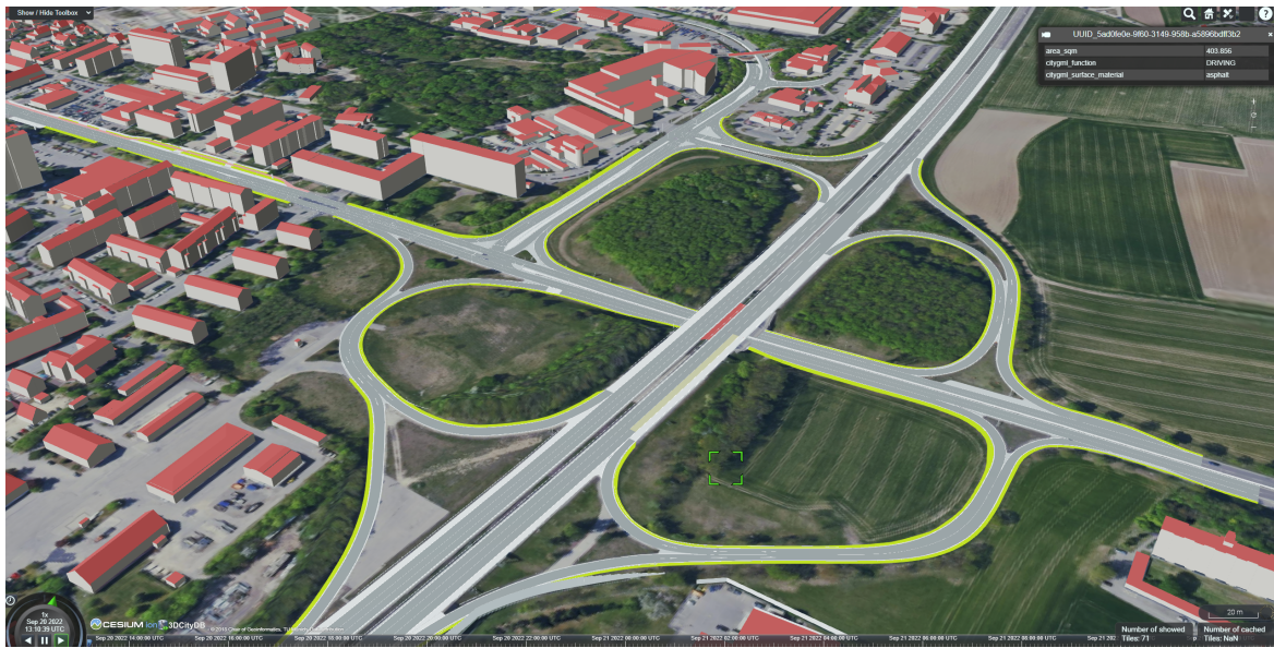
Figure 6.2: CityGML 3.0 compliant interchange in Ingolstadt generated from OpenDRIVE data combined with LOD 2 building models and visualized in a Cesium based web-visualization.
