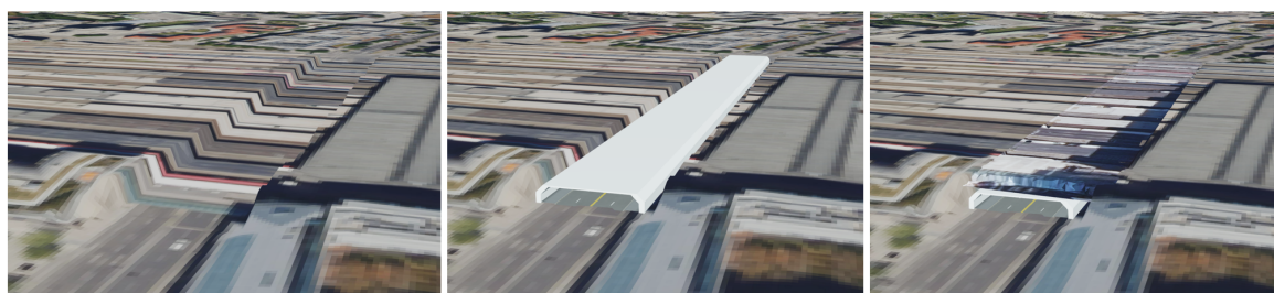
Figure 5.43: Visualization of a Tunnel containing road infrastructure underneath the terrain within Cesium. Left: Adapted terrain, middle: 3D road and tunnel model, right: added relief to close the adapted terrain model.
