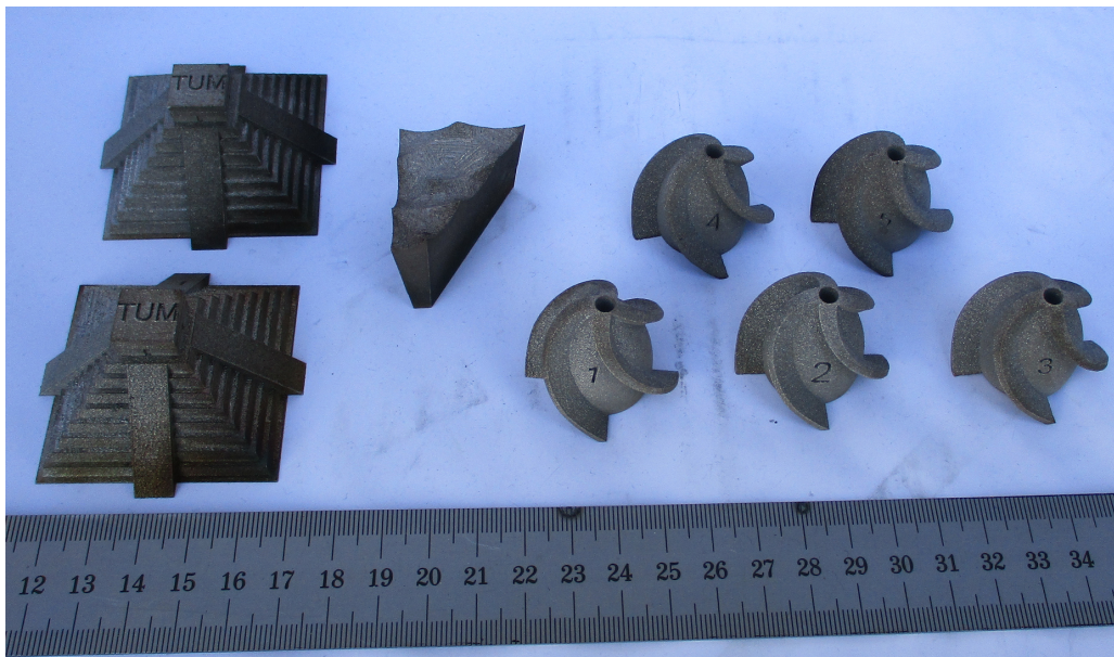
Figure 1 Specimens of the Buildjob E with five propellers, two pyramids and a model of the Elbphilharmonie .
