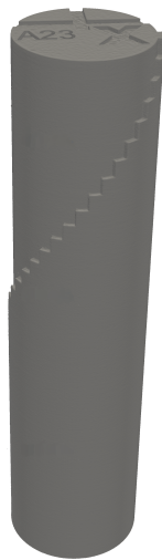
(a) Reconstructed CT volume with manually adjusted contrast for better visualization. In particular, the surrounding specimen holder is removed by manual adjustment.
