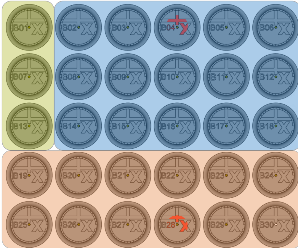
Figure 4.4 Buildplate of the Buildjob B with 30 specimens. The specimens are printed with varying focus (blue region) or decreased skywriting lead time (orange region). Additionally, reference specimens printed with standard parameters are marked in green.
