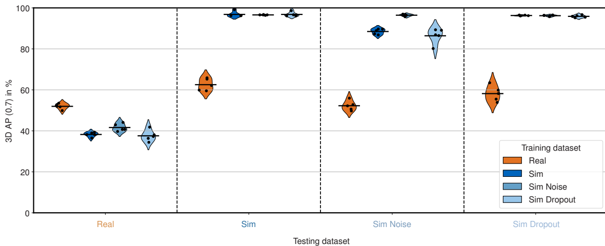
Figure 5.10: The 3D AP (0.7) for PointRCNN, which was trained and evaluated using either real , sim , sim noise , or sim dropout , data. The horizontal lines represent the mean AP and the five points represent the five individual training cycles for each training and testing combination (adapted from [213]).
