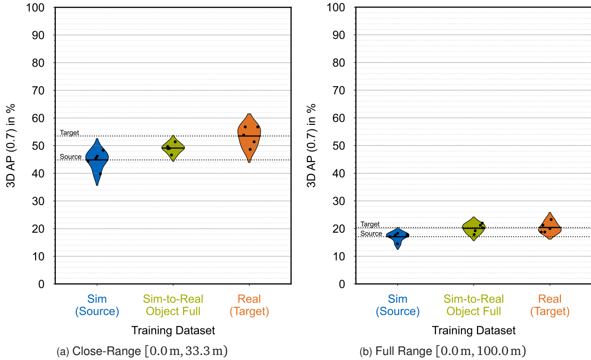
Figure 6.6: The 3D AP (0.7) for PointRCNN, which was trained and evaluated using either sim , sim-to-real object full , or real data and evaluated on real data (target). The horizontal lines represent the mean AP and the five points represent the five individual training cycles for each training and testing combination (adapted from [223]).
