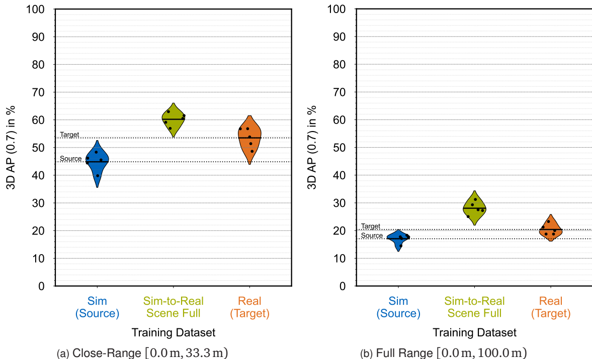
Figure 7.4: The 3D AP (0.7) for PointRCNN, which was trained and evaluated using either sim , sim-to-real scene full , or real data and evaluated on real data (target). Horizontal lines represent the mean AP and the five points represent the five individual training cycles per training and testing combination.
