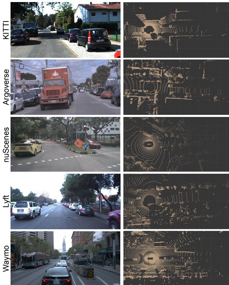
Figure 3.2: Front-view images (left) of five datasets and their corresponding LiDAR point clouds (right). The datasets are not only recorded in different geographic locations but also used different LiDAR sensor models to record the point clouds (from [106]).
