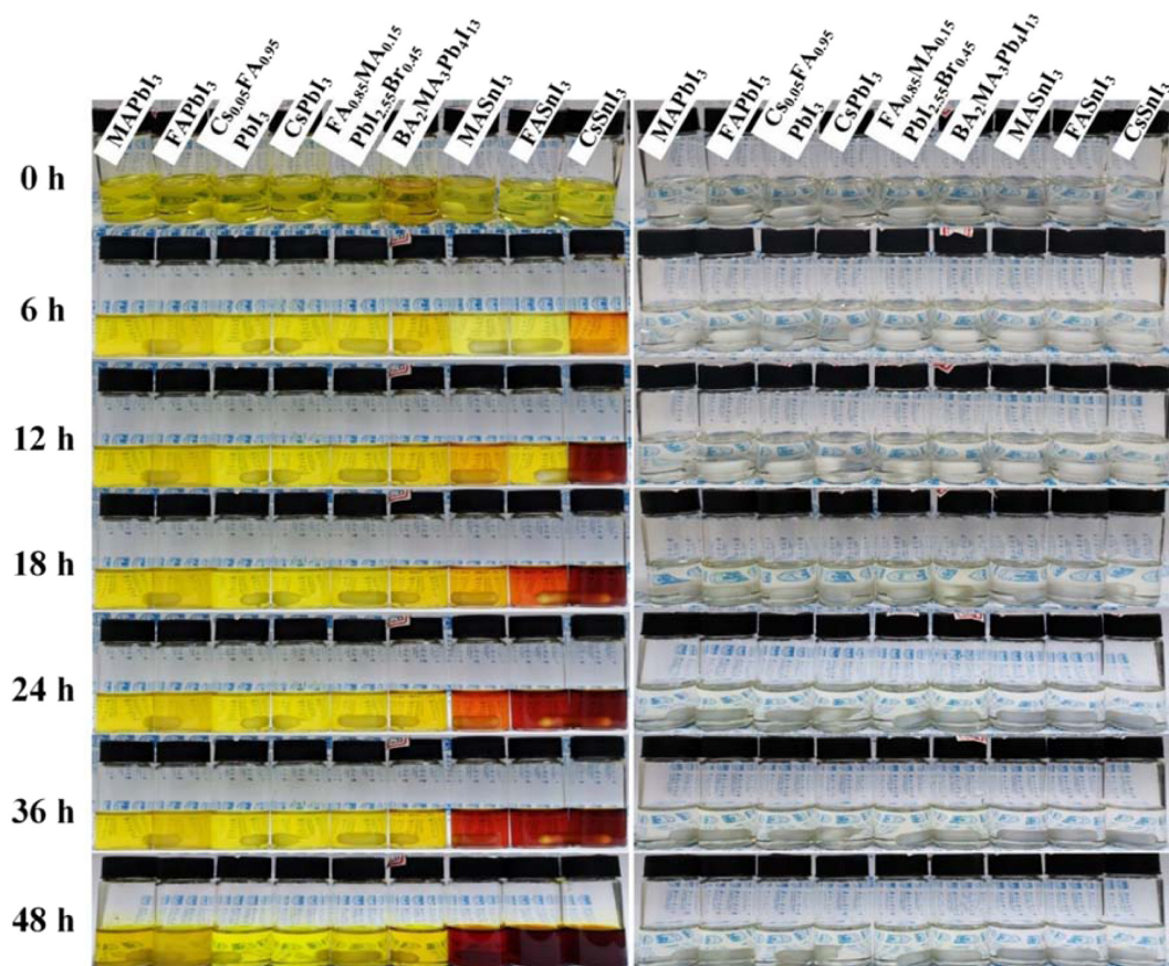
Figure 1 | Perovskite colloids precursor solution behaviors of traditional solvent and PIL. Photographs of the perovskite precursor solutions with different compositional precursors ( \text{MAPbI}_3 , \text{FAPbI}_3 , \text{Cs}_{0.05}\text{FA}_{0.95}\text{PbI}_3 , \text{CsPbI}_3 , \text{FA}_{0.85}\text{MA}_{0.15}\text{PbI}_{2.55}\text{Br}_{0.45} , \text{BA}_2\text{MA}_3\text{Pb}_4\text{I}_{13} , \text{MASnI}_3 , \text{FASnI}_3 , and \text{CsSnI}_3 ) in either MAAc (right) or DMF/DMSO (left) solvents with continuous aging in ambient environment.
