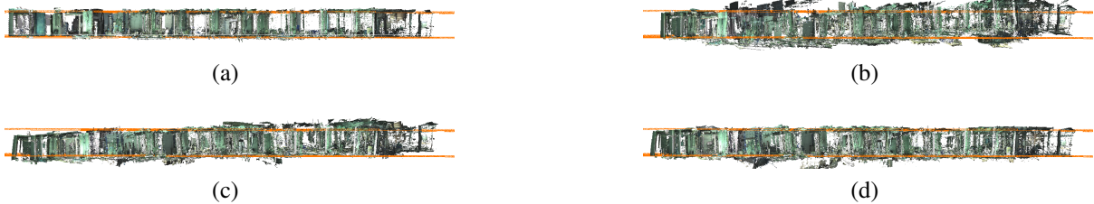
Figure 7: Side views of the different maps. (a) ground truth map; (b) map created with synthetic poses of Exp. 1; (c) map after FACaP optimization and (d) after BIMCaP optimization. The BIMCaP result shows better alignment with the real floor and ceiling planes.
