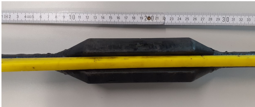
Figure 6-1. Downhole cable configuration of the sucker rod with a centralizer (black) and the fiber-optic cable (yellow).
