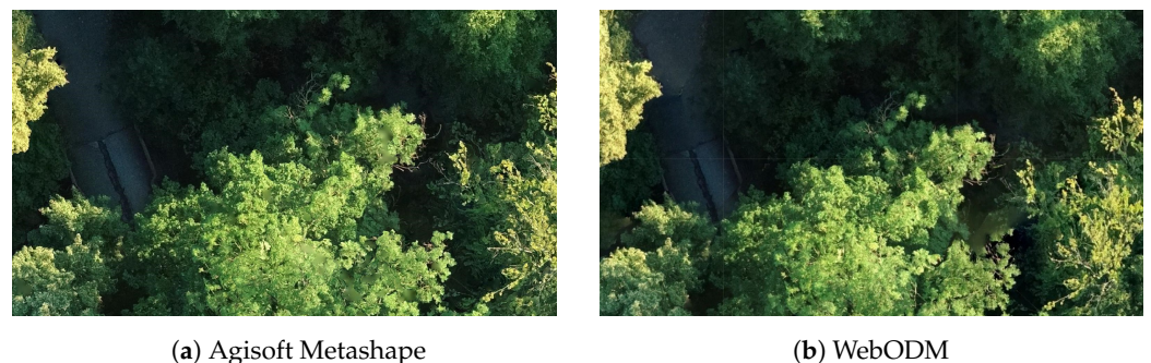
Figure 3. Comparison of the resulting orthomosaics and artifacts. Figure (a) shows artifacts from the orthomosaic generation with Agisoft Metashape, whereas (b) shows artifacts from the orthomosaic generation with WebODM.
