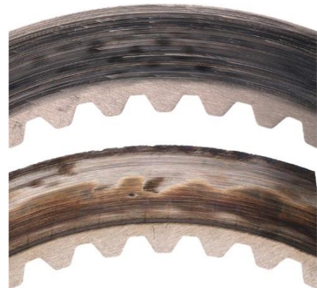
Figure 2.9: Local discoloration and sinter carryover on the steel plate for sinter friction systems [Sch20a].
