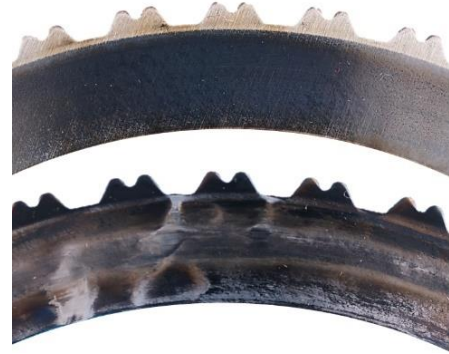
Figure 2.10: Local discoloration and local thickening on the steel plate for paper friction systems [Sch20a].
