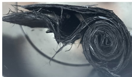
Fig. 5-7 Spiral charge showing the recurring separation between inner and outer layers of fibers within the sheet
