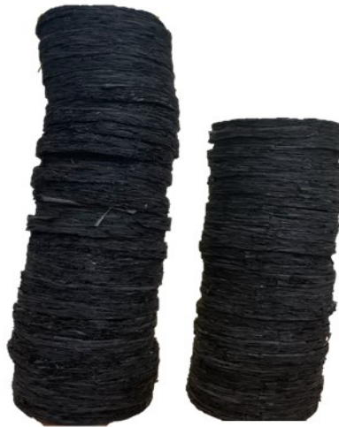
Fig. 5-9 Two disc pile charges with 28 discs with different heights due to varying sheet thickness
