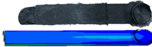
Fig. 3-30 Specimens resulting in the bar flow experiment and the simulation.
