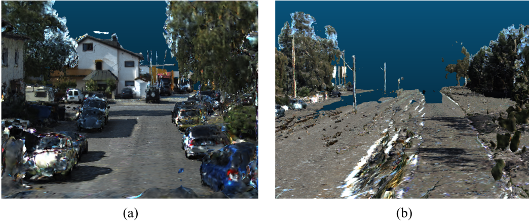
Figure 3.7: Mesh result reconstructed from KITTI dataset with no dynamic removal preprocessing applied in these two sequences. (a), KITTI-residential-0035; (b) KITTI-road-0015.
