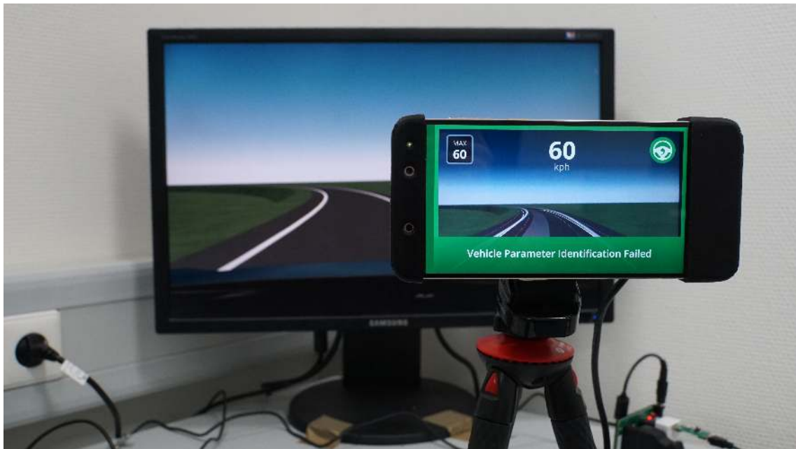
Figure 5.6: A view on our Hardware-in-the-loop setup, showing the EON (the smartphone in the front) and the carmaker simulation (the monitor in the back) running a concrete scenario.
