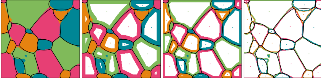
Figure 4.6: APDs for different degrees of grain scan-based interior removal (from left to right: none, and \bar{\delta} = 10, 6, 2 ). Shown are the computed diagrams (cell boundaries in black) based on the decreasing image supports (the non-white and non-black colored pixels in the respective images).
