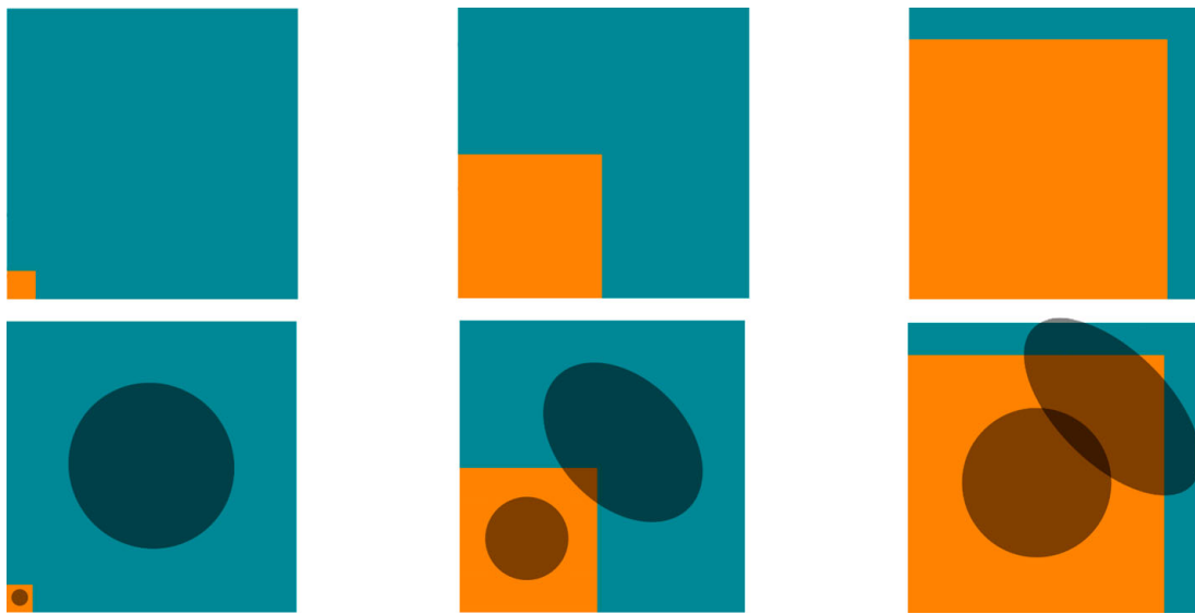
Figure 1. A family of grain scans involving a parameter \beta to illustrate differences between H1 and H2. Top, from left to right: Grain scans for \beta = 0.1 , \beta = 0.5 , and \beta = 0.9 . Grain G_1 (orange [light gray]) fills the square [0, \beta] \times [0, \beta] , G_2 (blue [gray]) fills the rest of the unit square. The bottom row shows the computed ellipses c_i + \mathbb{B}_{A_i}^2 with A_i = (\Sigma(G_i))^{-1} for i = 1, 2 .
