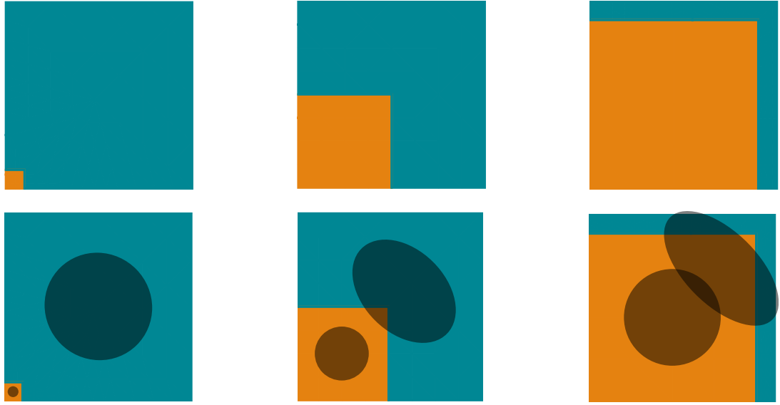
Figure 5.1: A family of grain scans involving a parameter \beta to illustrate differences between H1 and H2. Top, from left to right: Grain scans for \beta = 0.1 , \beta = 0.5 , and \beta = 0.9 . Grain G_1 (orange) fills the square [0, \beta] \times [0, \beta] , G_2 (blue) fills the rest of the unit square. The bottom row shows the computed ellipses c_i + \mathbb{B}_{A_i}^2 with A_i = (\Sigma(G_i))^{-1} for i = 1, 2 .
