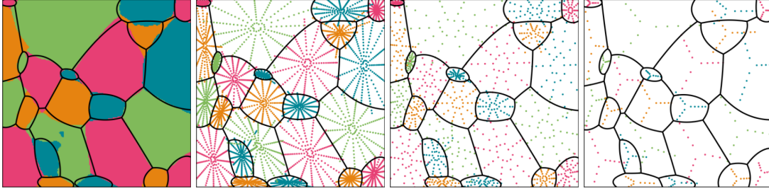
Figure 4.2: APDs from pencil coresets. From left to right: Computed diagrams (cell boundaries shown in black) based on decreasing image supports (the non-white and non-black colored pixels in the respective images). The diagram in the left image uses the full image support (the full available data), while the others use image supports living on pencils of decreasing density.
