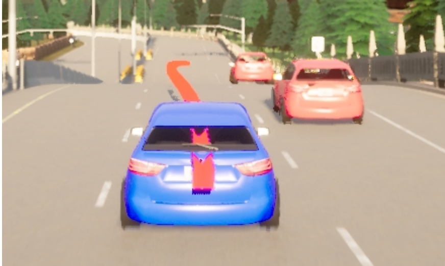
Figure 4.20.: Planned trajectory of the EV using the novel IMM+SMPC algorithm at time t = 4.80 s in the scenario in which TV2 eventually does not execute the lane change. © 2023 IEEE.
