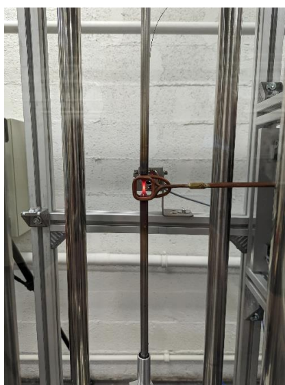
Figure 1 : Ultrasonic fatigue machine and inductive specimen heating system
