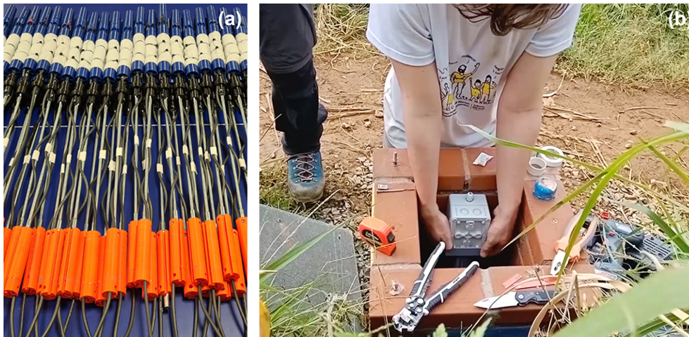
Figure 10. (a) Sensor probes ready for installation. The piezometer (blue) is located at the bottom of the probe. Above this follows a ball joint (black) which exactly fits into the used installation pipes and functions as a reference point for the inclination measurements. Then comes the first inclination sensor (orange), which – when installed – is followed by another ball joint (second reference point located exactly 1 m above the first joint). If required, further inclination sensors can be added. (b) Installation of subsurface probe into a brick seating cube.
