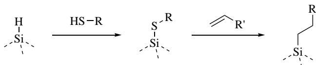
Scheme 5.8: Schematic description of the thiolation of silicon atoms in silicon nanocrystals and subsequent ligand exchange of the thiolated material by the reaction with an alkene.
