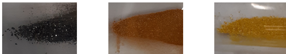
Figure 2.3: Photographs of germanane, gersiloxene with Ge/Si = 1:1, and silicane (from left to right).
