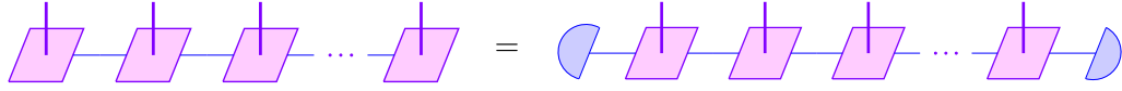
Figure 1.16: MPS with open boundary conditions, where boundary tensors that have one index fewer may be constructed by acting upon the dangling boundary indices with appropriate vectors, shown in blue.
