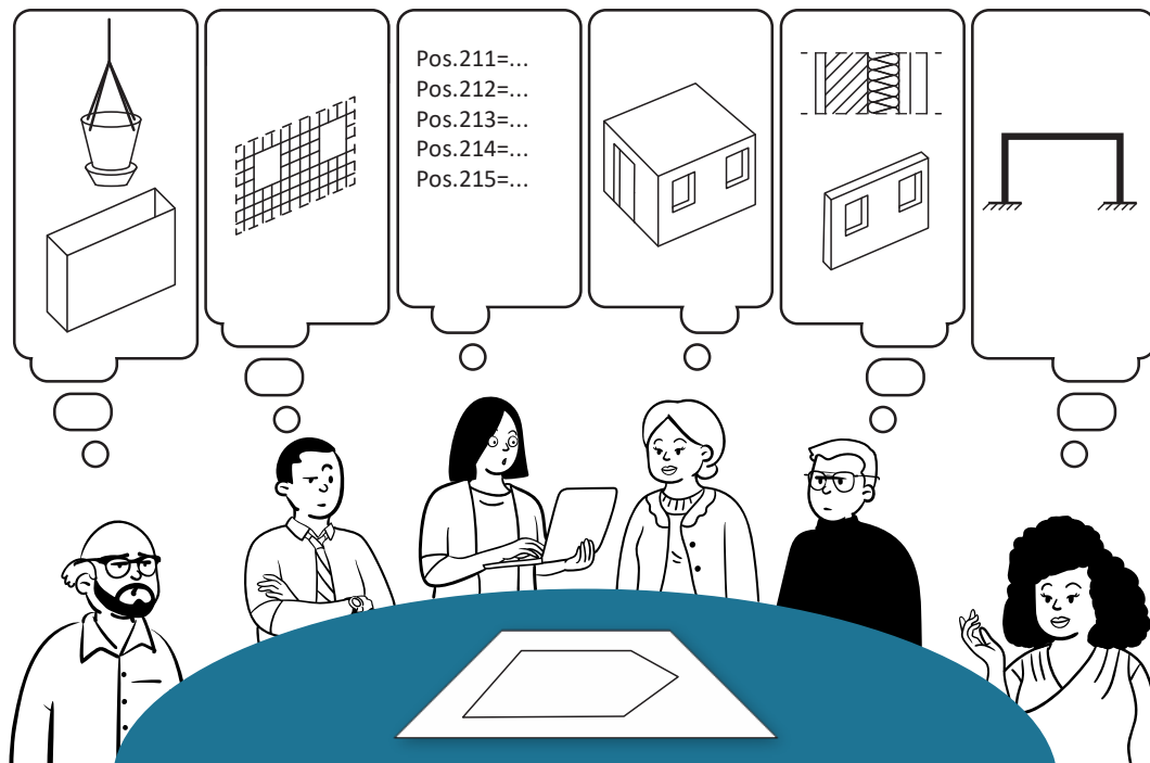
Figure 1 - Different interpretations of the same design among parties involved in the planning and construction based on (Junge and Liebich 1997)
