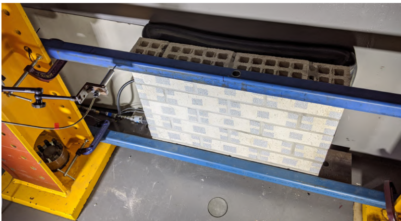
(b) Bending test setup with direction e_1 masonry sample.
