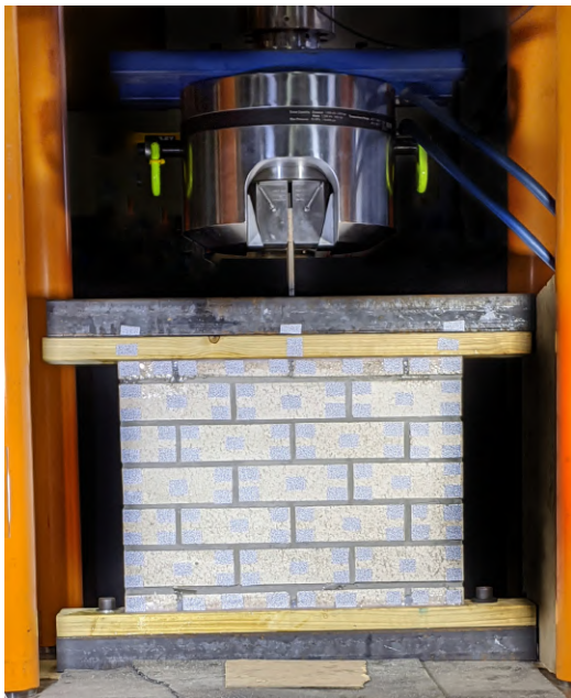
Figure 4.15: Tensile test setup with horizontal brick specimen.
