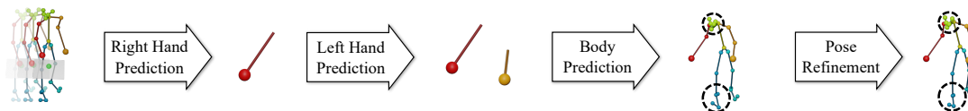
Figure 3.4: To model joint dependencies within the human skeleton, we sample joints in an autoregressive manner by first predicting the end-effectors (right and left hand), then the rest of the body; pose refinement then improves skeleton consistency.
