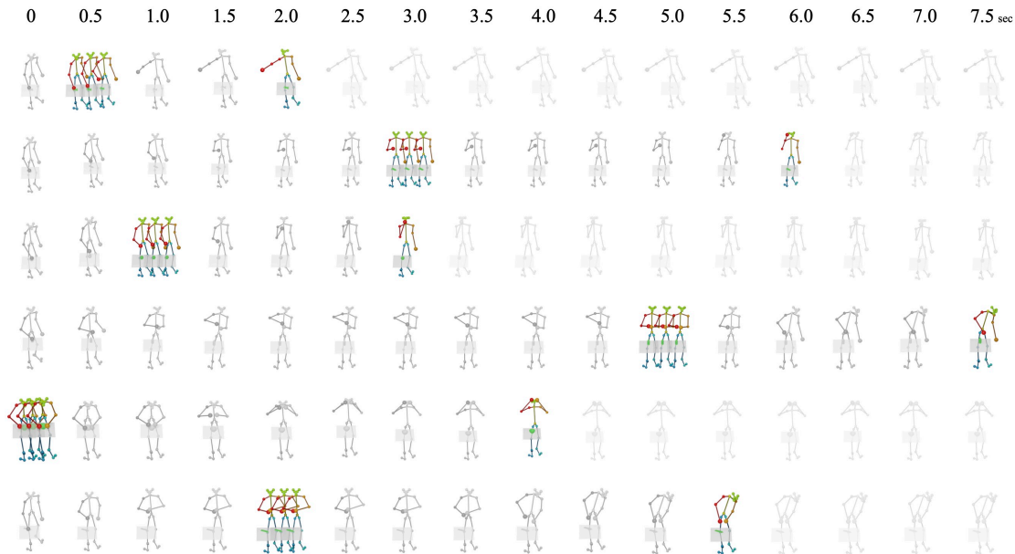
Figure 3.12: Sample input-target pairs (colored) for our characteristic 3D pose forecasting task, with temporal snapshots along the sequence (grayscale). Each snapshot is half a second apart. Depicted as input is the last frame of the respective input sequence.
