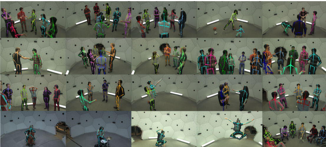
Figure 2.12: Specialized multi-camera setup for capturing human motion, e.g., the human motion capture dome for the CMU Panoptic Dataset [60].
