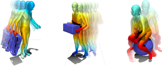
Figure 3. An object’s trajectory is largely defined by the motion of the region of the body in close contact with the object, e.g. the hand(s) when carrying an object (left, middle) or the lower body when moving with an object while sitting (right). This informs our contact-based approach to generating object motion.
