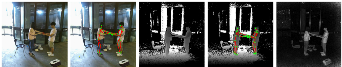
Figure 2.11: Human motion capture using monocular depth data, as used in the NTU RGB-D dataset [56, 57]. From left to right: RGB color image, overlaid detected poses in 2D, depth as captured by the sensor, joint detections from RGB transformed and overlaid on top of the depth image, and the infrared image captured by the sensor.
