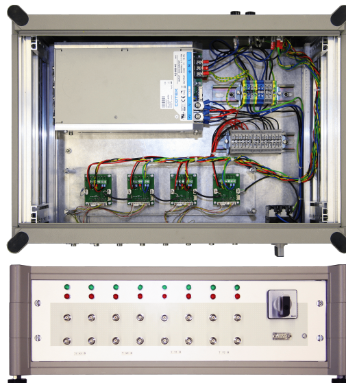
Figure 19.9: Top and front view of the built amplifier. Top: Power supply in the top left corner and 2 stacks with each 4 current controller.
