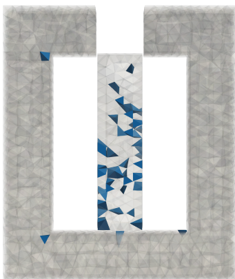
(a) pECSW selected elements are located in the ferromagnetic materials. A higher density of elements is found in the target body, which undergoes a higher magnetic flux density.
