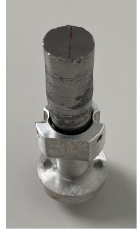
Figure 2.11: Panel a: Magnetic phases of MnSi as a function of temperature and external magnetic field, as determined by ultrasonic studies conducted by A. Bauer et al. [99]. Panel b: Photo of a cylindrical MnSi sample mounted on an aluminium sample holder. The red line indicates the [011]-direction aligned using the ORION instrument at the Swiss spallation neutron source SINQ, PSI, Villigen, Switzerland.
