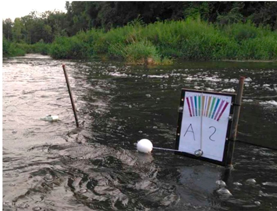
Figure 3. Installed Surface Roughness Measurement Device (SRMD) on a pole and a small float with temperature logger in the fluvial mesohabitat type (FMH) pool.
