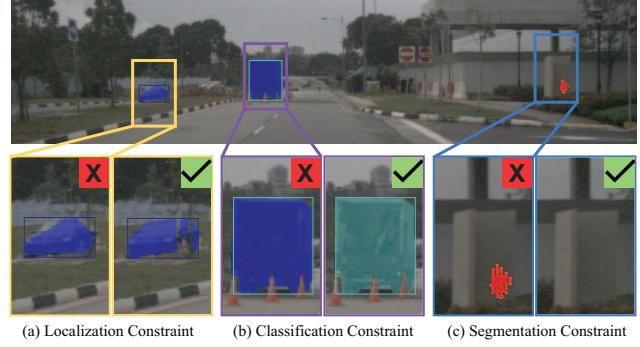
Figure 1: Consistency constraints between object detection and semantic segmentation. (a) Segmentation mask covers all pixels of a detected object. (b) A detected object and the segmentation mask that covers it share the same predicted class distribution. (c) No pixels outside of the detected boxes are segmented with an object class.
