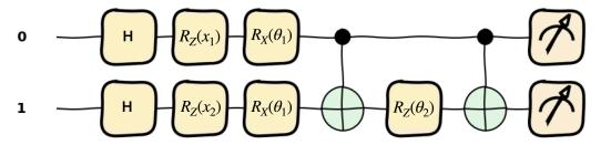
**Figure 5.** Illustration of the quantum circuit used for EQNN at depth 1. This circuit is repeated five (ten) times with different parameters for the symmetric (anti-symmetric and fully anti-symmetric) case. The data points  $(x_1, x_2)$  are loaded via angle embedding with two  $R_Z$  gates,  $R_Z(x_1)$  and  $R_Z(x_2)$ . The remaining circuits are parameterized by  $R_X(\theta_1)$  and  $R_Z(\theta_2)$ .
