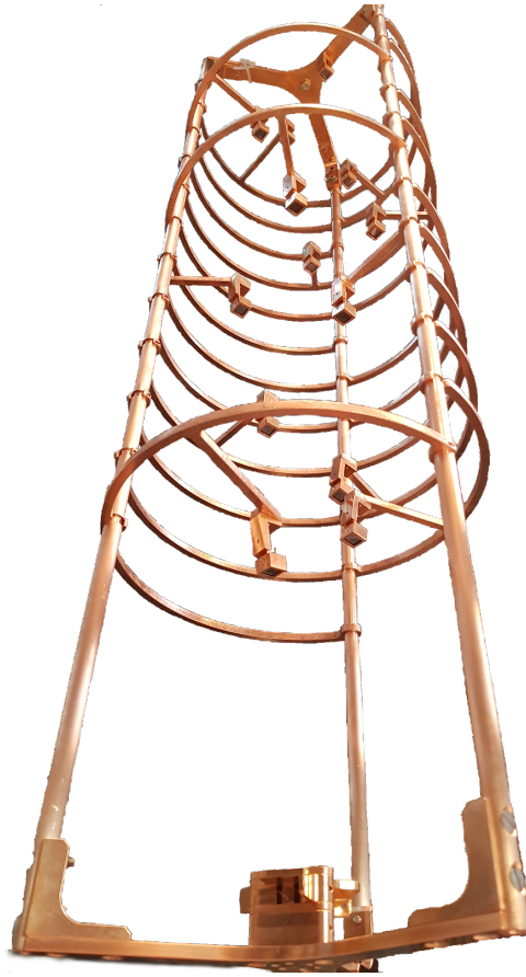
Figure 5.1: The LLAMA instrument. A cylindrical copper frame holds 13 SiPMs in distances from 15 cm to 75 cm in steps of 5 cm to a light source, which is mounted on the bottom plate (see fig. 5.2). Individual transversal displacements prevent shadowing, and each SiPM faces the light source directly.
