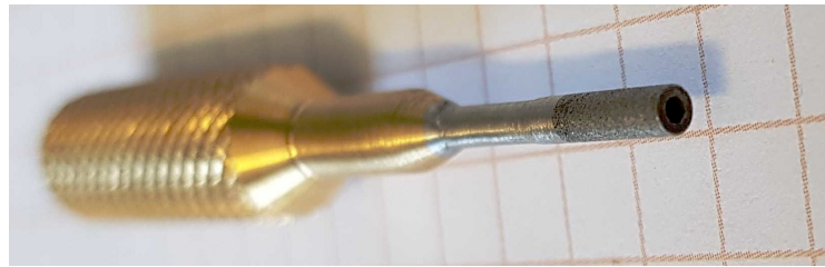
Figure B.5: Manual mechanical cleaning device featuring a diamond milling head at its tip. The milling head has been used since the 2nd cleaning campaign. Its hollow center fits over individual pins of the socket.
