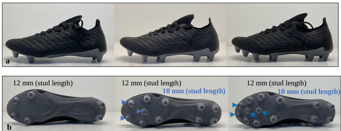
Figure 4.3.1.a Three-dimensional printed (outsoles of ) boots, side view (upper photo). b Outsole configuration with different stud lengths (those shown with the arrow are 10 mm in length, and the rest are 12 mm in length)
