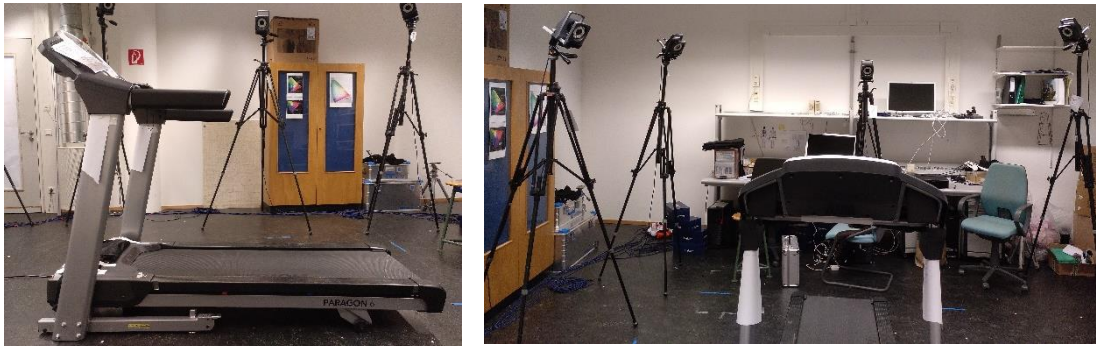
Figure 2.3.2 Positions of the number of Vicon cameras on the day of the experiment
