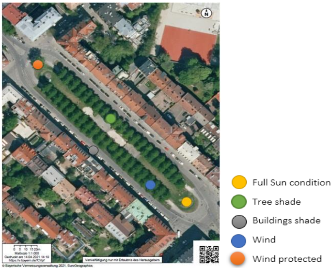
Figure 18 Top-View Bordeauxplatz, location of i-Buttons devices, P.Stark [87]
