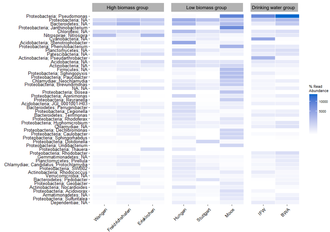
Figure 9.3. Taxonomic composition of eight sand filters at the phylum and genus level revealed by the most abundant 50 ASVs.
