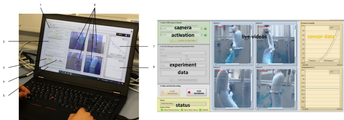
Figure 9. Human machine interface during an experiment. The figure displays the HMI on a laptop used during the experiment. 1 = Camera activation: allows the user to activate the cameras for recording; 2 = Enter experimental data: enables inputting relevant experimental data; 3 = Start recording
