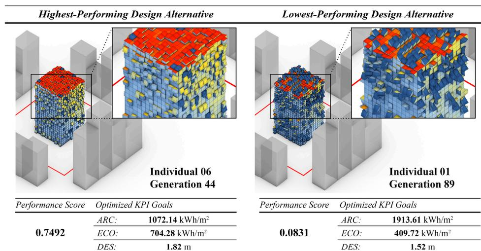
**Figure 6.** Comparison between the highest- and lowest-performing optimized design alternatives. Solar radiation values are depicted from the lowest (blue) to the highest (red) values. The figures were previously published in (Selvan et al. 2023) [69].
