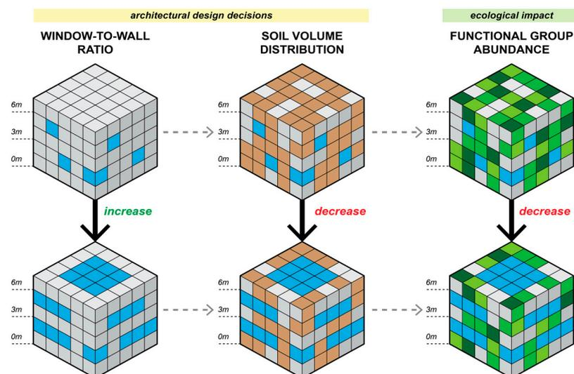
**Figure 5.** A schematic example of the architectural geometry of the building envelopes in relation to floor height and surface openings (windows—blue colour), as well as the soil volume (brown colour) and FG abundance (green colour).
