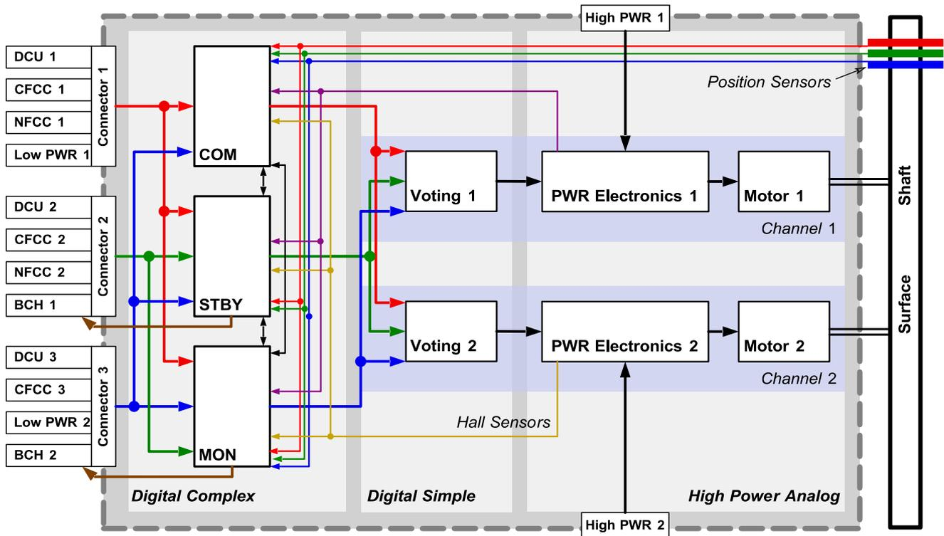
DCU: Data Concentrate Unit    NFCC: Nominal Flight Control Computer    CFCC: Critical Flight Control Computer
