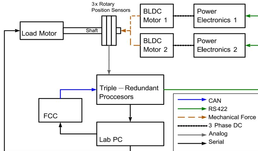
Figure 7. VoDeMo test bench schematic.
