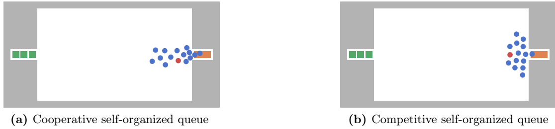
Figure 7.7: The snapshots of two simulations demonstrate how the waiting crowd (susceptible – blue, infectious – red) forms a self-organized queue in front of a service unit (orange rectangle). Queue management strategies are not explicitly applied. Note: own figures adapted from [213, p. 3].
