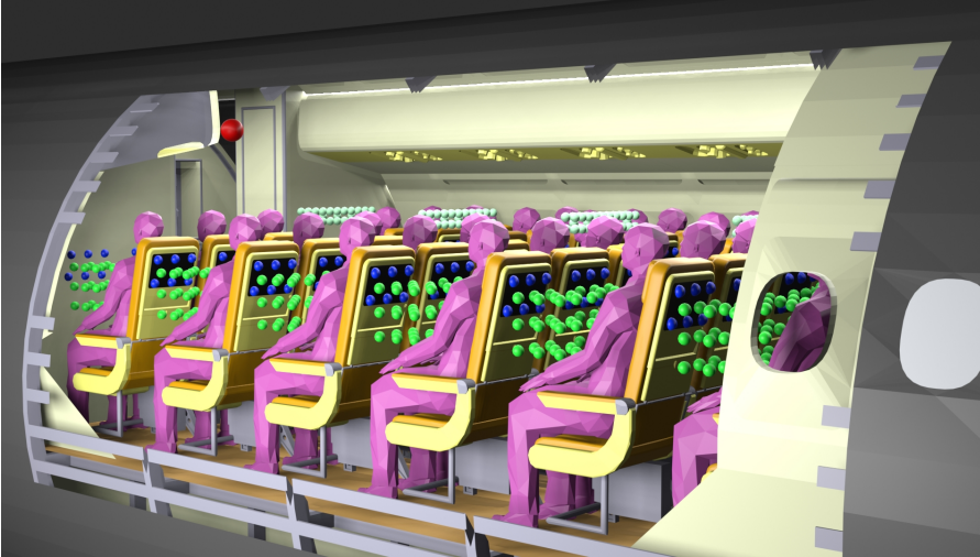
Figure 3.2 Transmitter and receiver positions in the cabin. Red: Tx0, Cyan: Receiver Aisle, Blue: Receiver Screens, Green: Receiver Seats
