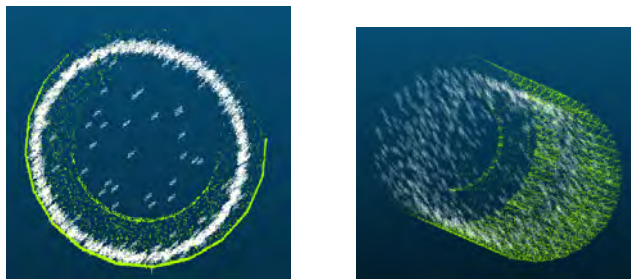
Figure 4.4: Overlaying Input (green) and Output (white) of DuctSilencer Testing instance (front and side)
