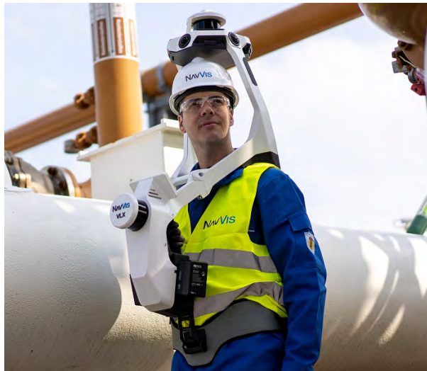
Figure 3.8: NavVis VLX 3 worn by a person (GOGEOMATICS NEWSMAKERS, 2023)
