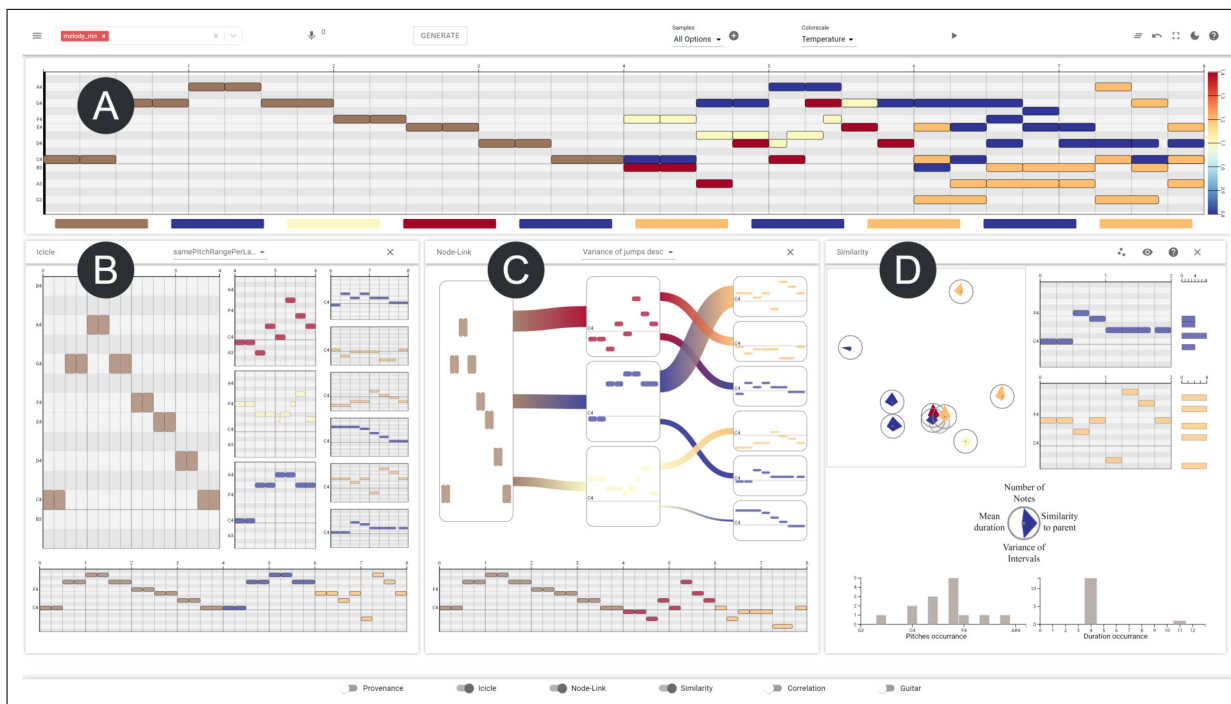
Figure 1. Overview of our design: (A) Piano roll to show/edit the composition. (B) Icicle plot and (C) node-link chart for tree structures. (D) Similarity-based scatterplot as overview of all samples. Color encodes the AI’s temperature parameter.
