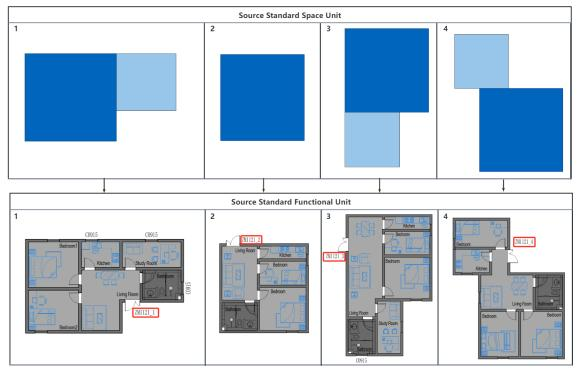
Figure 5.5 Configuration of all source standard functional units
