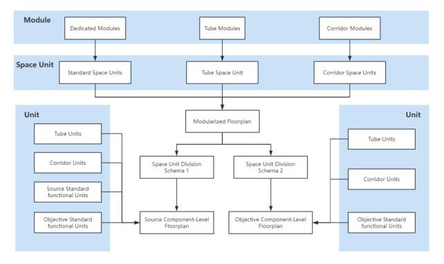
Figure 3.1. Modularized Design Process for Prefabricated Frame-Tube Structures
