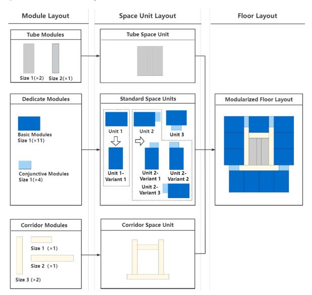
Figure 3.6. Modularized Floor Layout Configuration Process
