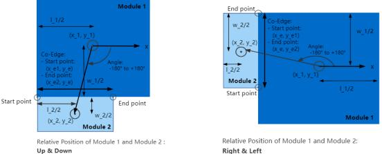
Figure 4.7. Connectivity between Module 1 and Module 2 under the 4 Kinds of Relative Positions
